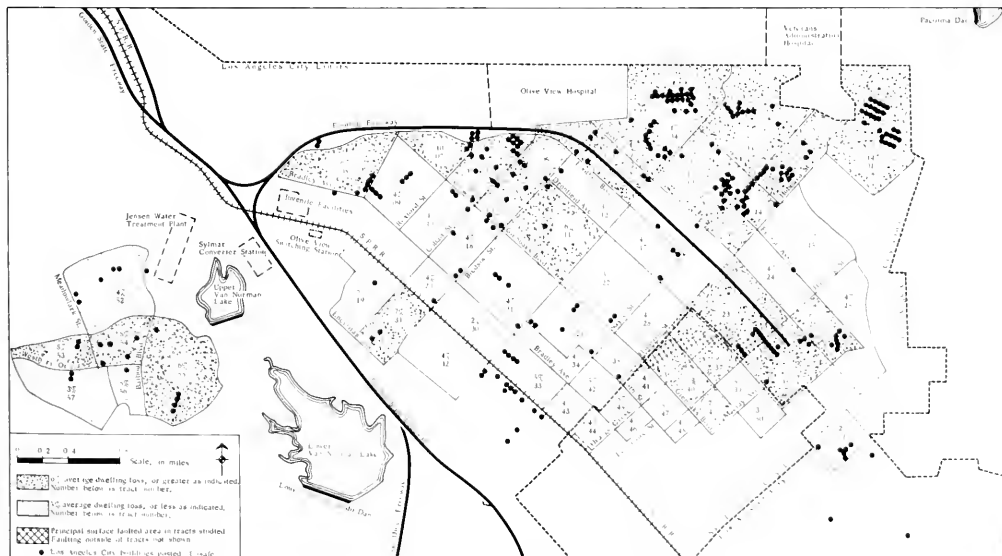
Figure 5. Map showing the distribution of damage with special reference to wood frame dwellings.
